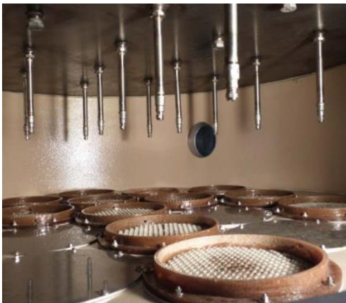
Figure 4-2 HeatMatrix exchanger equipped with an in-situ cleaning system
