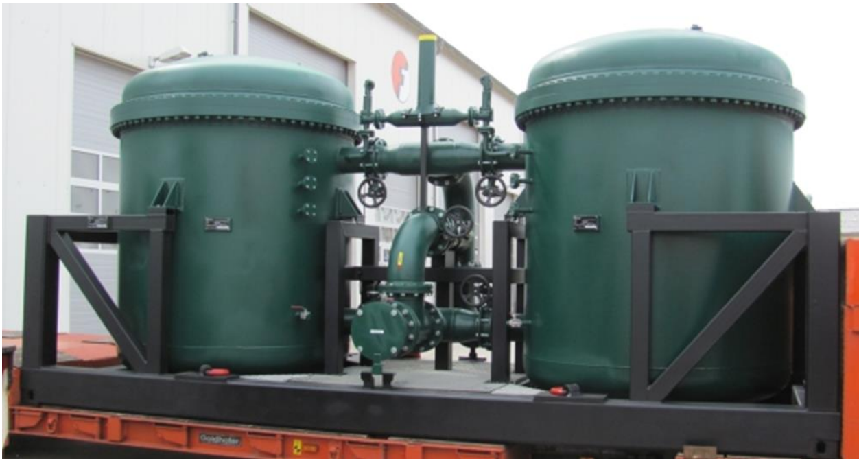
Figure 14: Example Fangmann Industrie – separator skid with two adsorbers (DN 250; DP64)
