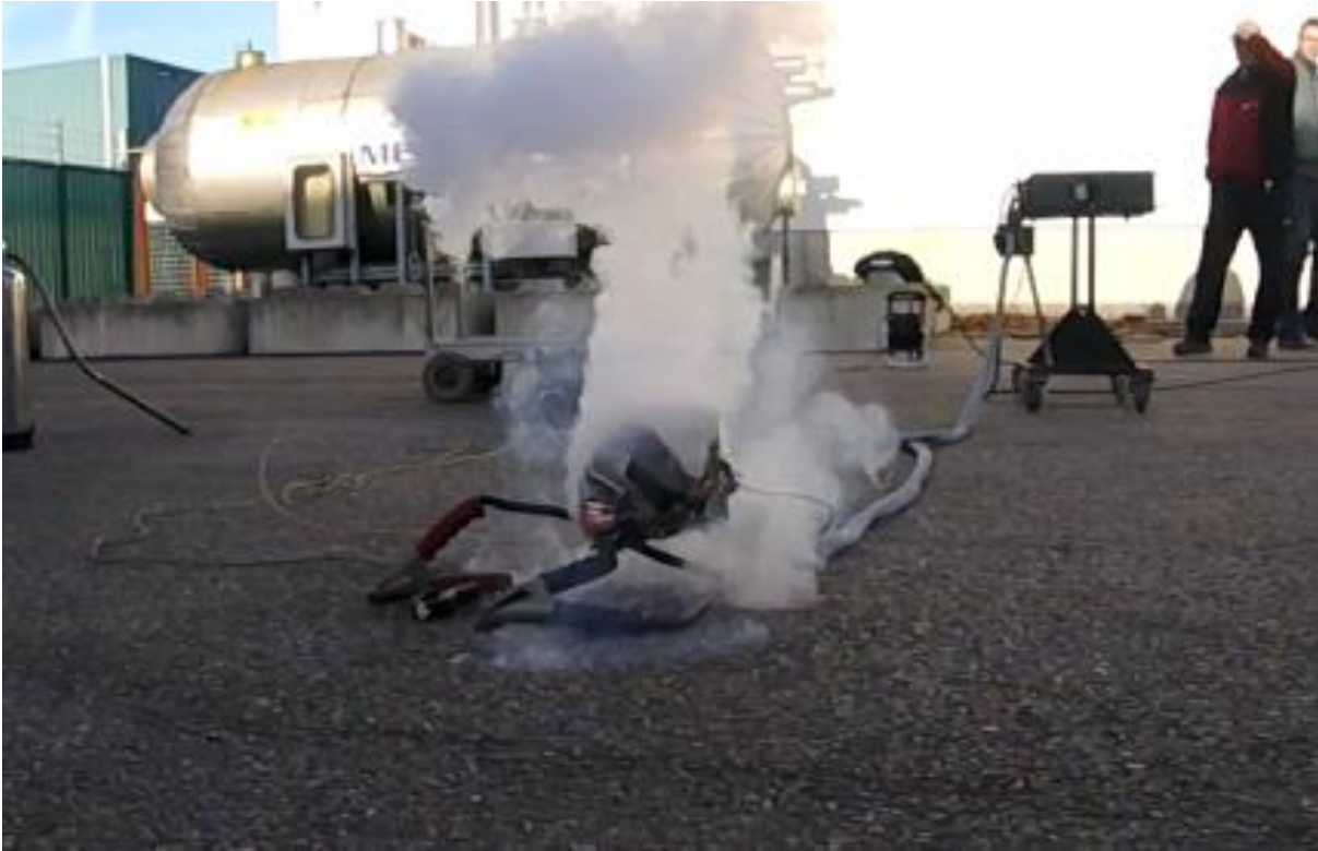
Figuur 10. Cel 1 scheurt open
