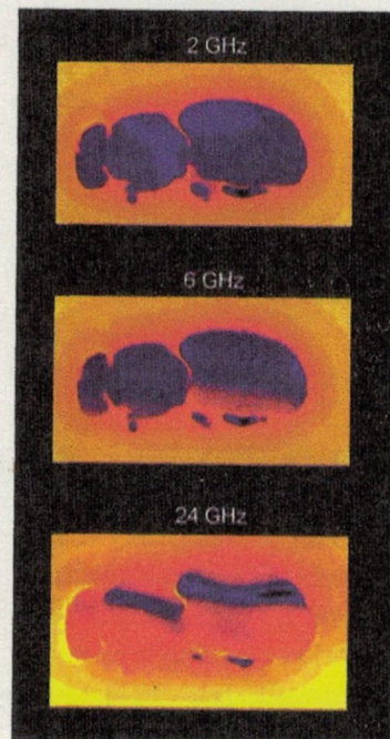
FIGURE 5. Illustration of the absorption of Radio Frequency electromagnetic radiation in the Honey Bee. At currently used frequencies between 2 GHz (top) and 6 GHz (middle), the wavelength is relatively large compared to the insect. But at 24 GHz, (bottom) the wavelength is closer to the insect's size and the radiation penetrates further. 7
