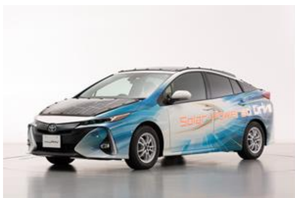
Fig. A-3 PV-powered Prius-HEV (Toyota) ( https://www.nedo.go.jp/news/press/AA5_101150.html )
