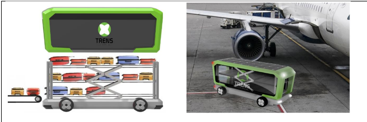
Figure 12. Solar-powered luggage vehicle concept by J. Liao, N. Pizzigoni and V. Rachmanda.
