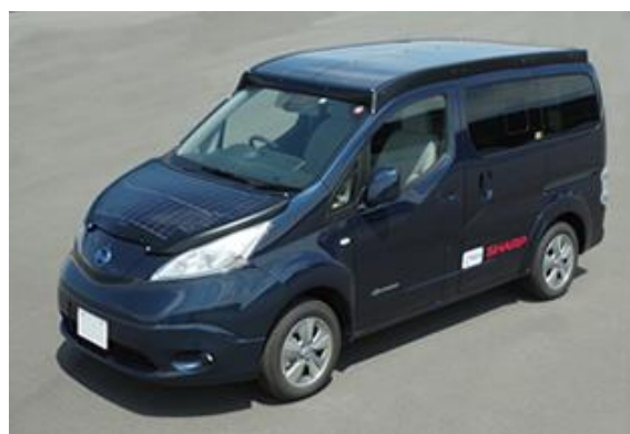
Fig. A-4 PV-powered e-NV200 (Nissan) ( https://www.nedo.go.jp/news/press/AA5_101326.html )
