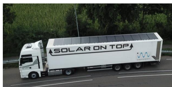
Fig. B-2 PV truck trailer (Photo: IM Efficiency)
