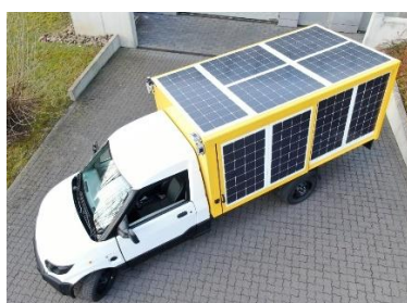
Fig. B-1 PV-powered light commercial vehicle (Photo: Institute for Solar Energy Research Hamelin)
